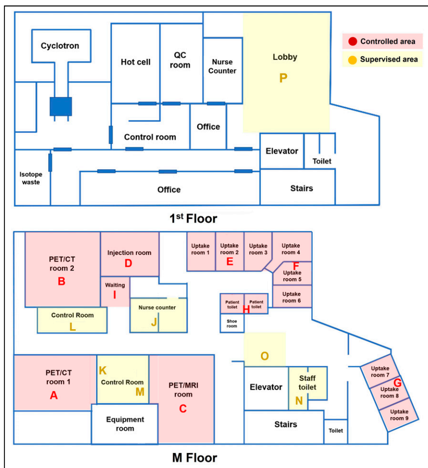
FIGURE 2. Floor plans for first floor and M floor of National Cyclotron and PET Centre at Chulabhorn Hospital. QC = quality control.
