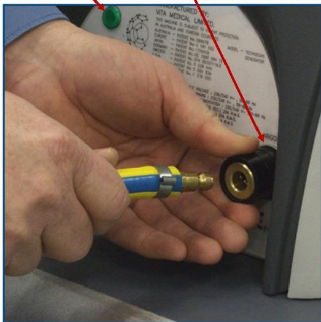
Figure 2: Annotated rear view of the Technegas generator demonstrating connection of argon to the system (image courtesy of Cyclomedica).
