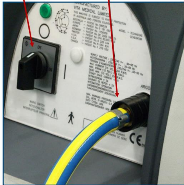
Figure 2: Annotated rear view of the Technegas generator demonstrating connection of argon to the system (image courtesy of Cyclomedica).
