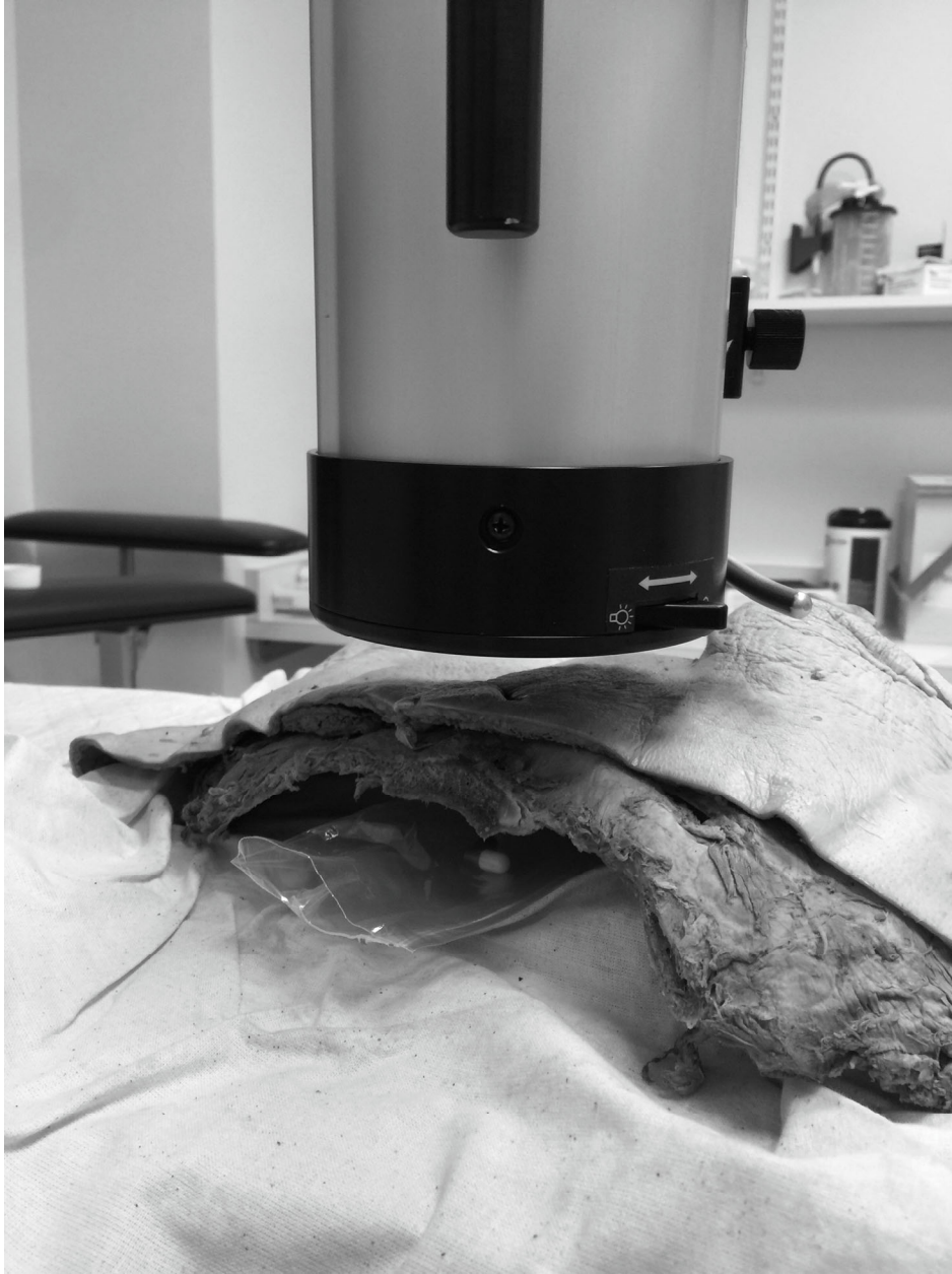
Figure 3. Demonstration of counting of the iodine capsule attenuated by a cadaveric chest wall. The image demonstrates the capsule (within a sealed plastic bag), below the chest wall. The thyroid probe is positioned 24 cm above the chest wall.
