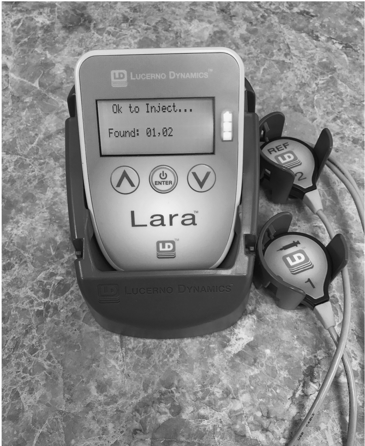
Figure 1: Modular detector device (Lara ®). The digital screen and two of the four detectors shown.
