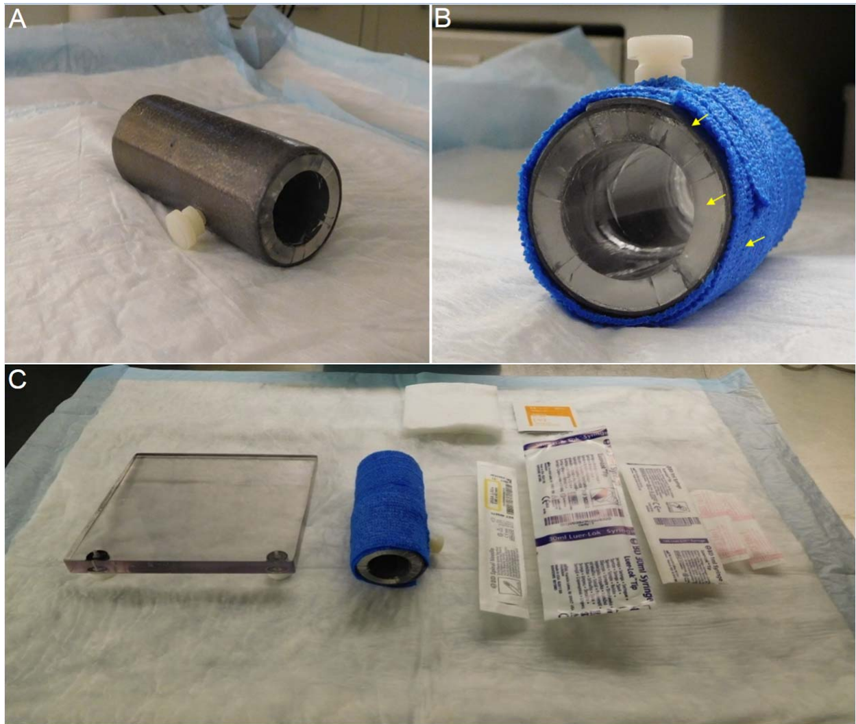
Figure 2 Dose Preparation Supplies. A. In-house fabricated 30-mL syringe shield. B. From outer to inner, arrows represent the covering to prevent contact with lead surface, lead, and acrylic. C. Some supplies needed to draw up the dose (a wedge, 30-mL syringe shield, gauze, alcohol wipes, 30-mL syringe, 3 1/2" spinal needle, 1-mL syringe, 20-gauge (g) needles, chux pad).
