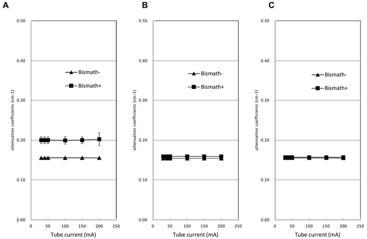
Fig. 4 Comparison of attenuation coefficients with and without bismuth shielding
