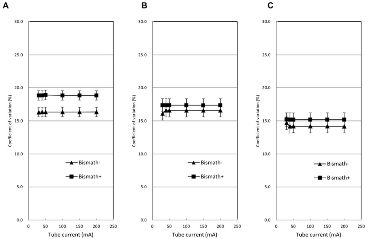
Fig. 5 Coefficient of variation as a function of bismuth shielding (A) Top, (B) middle, and (C) bottom of the image. Coefficient of variation = SD/mean
