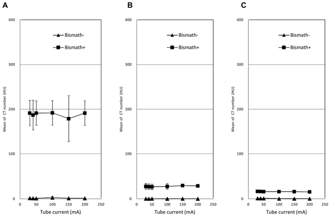
Fig. 3 Mean of CT number determined on CT images as a function of bismuth shielding
