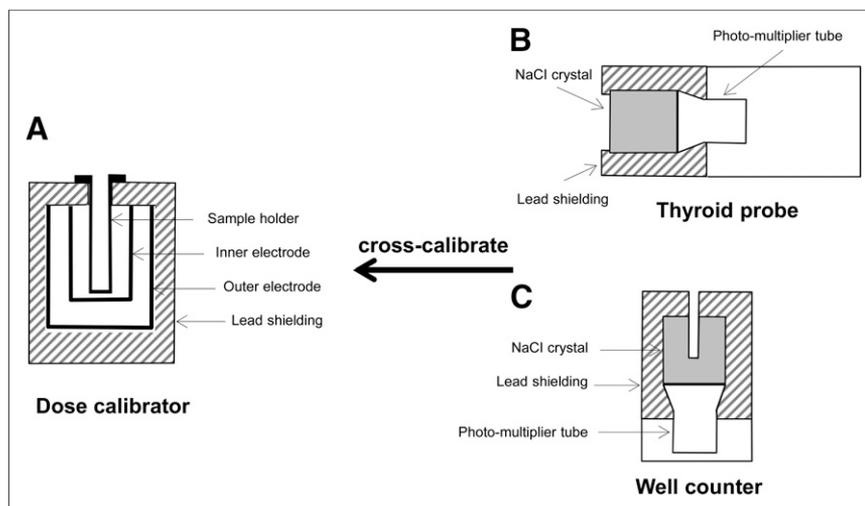
**FIGURE 1.** Cross calibration against dose calibrator (A) is needed to convert count readings from thyroid probe (B) and well counter (C) to units of activity (kBq or  $\mu\text{Ci}$ ) for blood samples.
