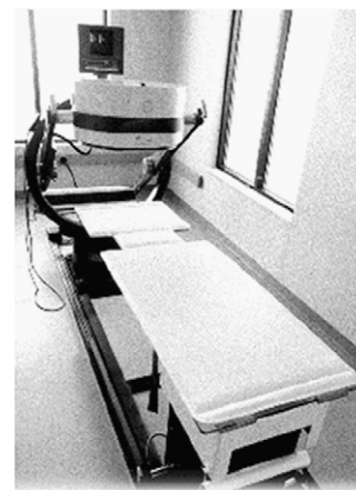
FIGURE 2. Large-field-of-view \gamma -camera with table modification for prone breast positioning.
