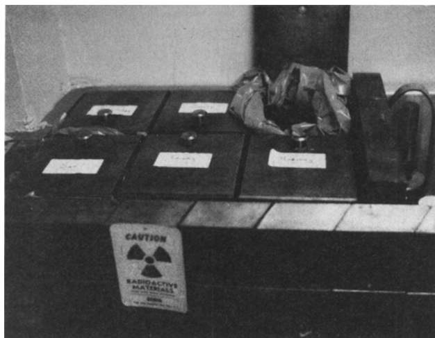
FIG. 1. Six chambered box for day-of-the-week storage of technetium.
