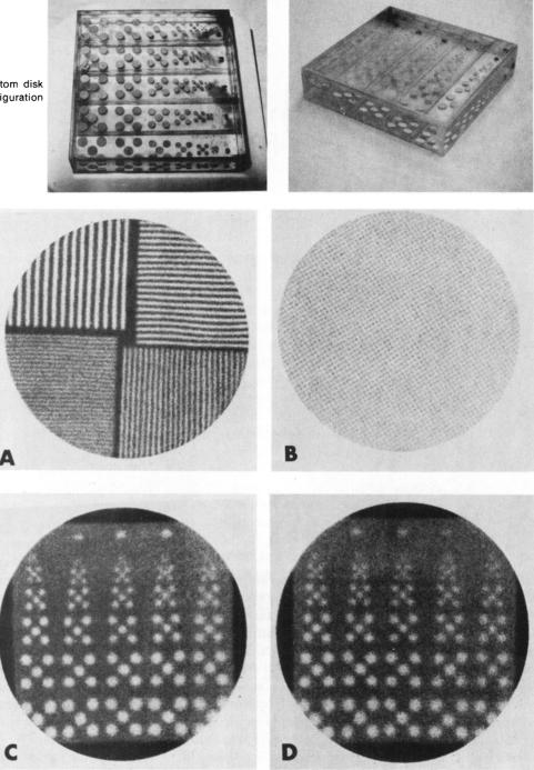
Fig. 2. (A) Standard bar phantom (1/4 in., 3/16 in., 1/8 in., 5/32 in.) obtained on the surface of the collimator of the Picker system. (B) Smith orthogonal hole phantom image obtained intrinsically (1/8 in. holes, 1/4 in. centers). (C) Phantom described imaged extrinsically representing 0.0-cm through 4.0-cm depth and (D) 3.0-cm through 7.0cm depth.
