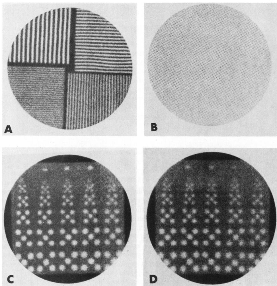
**Fig. 2.** (A) Standard bar phantom (1/4 in., 3/16 in., 1/8 in., 5/32 in.) obtained on the surface of the collimator of the Picker system. (B) Smith orthogonal hole phantom image obtained intrinsically (1/8 in. holes, 1/4 in. centers). (C) Phantom described imaged extrinsically representing 0.0-cm through 4.0-cm depth and (D) 3.0-cm through 7.0-cm depth.
