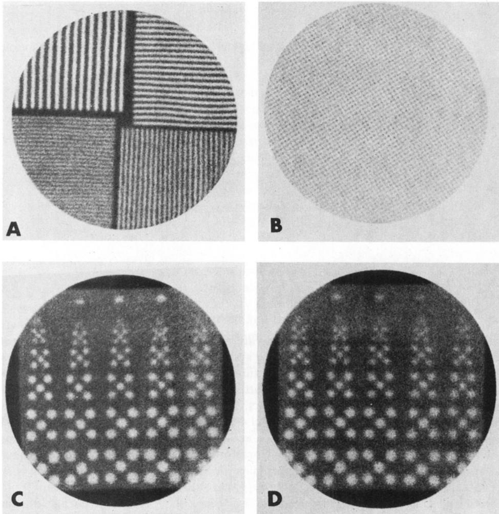
**Fig. 3.** Standard bar phantom (1/4 in., 3/16 in., 1/8 in., 5/32 in.) obtained on the surface of the collimator of the General Electric system. (B) Smith orthogonal hole phantom image obtained intrinsically (1/8 in. holes, 1/4 in. centers). (C) Phantom described imaged extrinsically representing 0.0-cm through 4.0-cm depth and (D) 3.0-cm through 7.0-cm depth.
