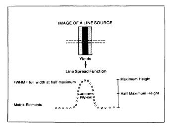
FIG. 2. Diagramatic representation of the line-spread function.
