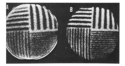
**FIG. 2.** (A) Comparison of intrinsic resolution of the Pho-Gamma III HP camera and General Electric Portacamera (B) using 20% window and a preset count of 600K. The bar phantom used consisted of alternating lead bars spaced a 1.25 cm, 0.95 cm, and 0.47 cm.
