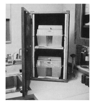
FIG. 5. Vault structure open reveals two shelves for current and previous week generators.
