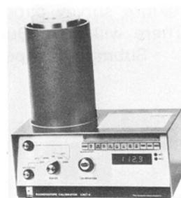
isotopes, the CRC-5 also provides over 90 radioisotope calibrators for manual selection. Available options include a remote calibration detector and a radiation exposure monitor.
