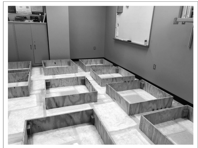
FIGURE 1. Absorbent pads and 0.28\text{ m}^2 ( 3\text{ ft}^2 ) plywood sample boxes ready for controlled ^{90}\text{Y} -RM spill.
