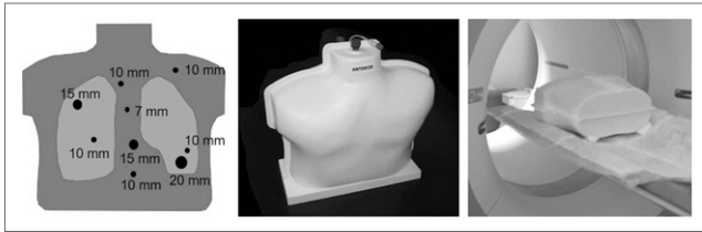
FIGURE 1. Anthropomorphic chest oncology simulator with 9 internal spheric lesions. Lesion locations and size are shown at left. Phantom positioned supine in scanner is shown at right.
