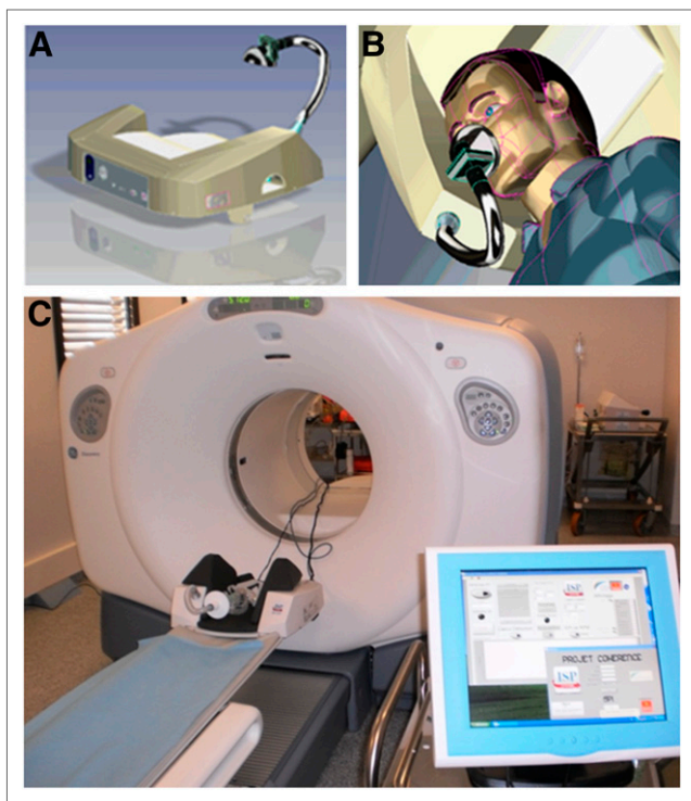
FIGURE 1. SGD PET/CT setup. (A) SGD device. (B) Patient positioning by computer-assisted design. (C) SGD device position on PET/CT camera with screen monitoring.
