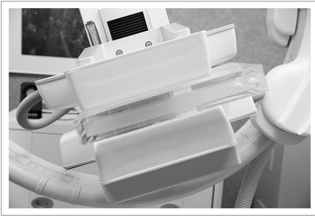
**FIGURE 2.** Proper positioning for uniformity flood acquisition using refillable  $^{99m}\text{Tc}$  source. Source is positioned between upper and lower detectors of dual-head cadmium-zinc-telluride system. Gantry is angled to ensure that any air bubbles in phantom are outside field of view.
