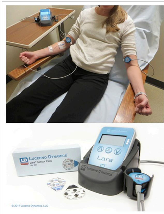
**FIGURE 1.** (Top) Sensors placed on injection arm and contralateral control arm. (Bottom) Lara device consists of 2 scintillation sensors, 2 pads, a reader, and a docking station.
