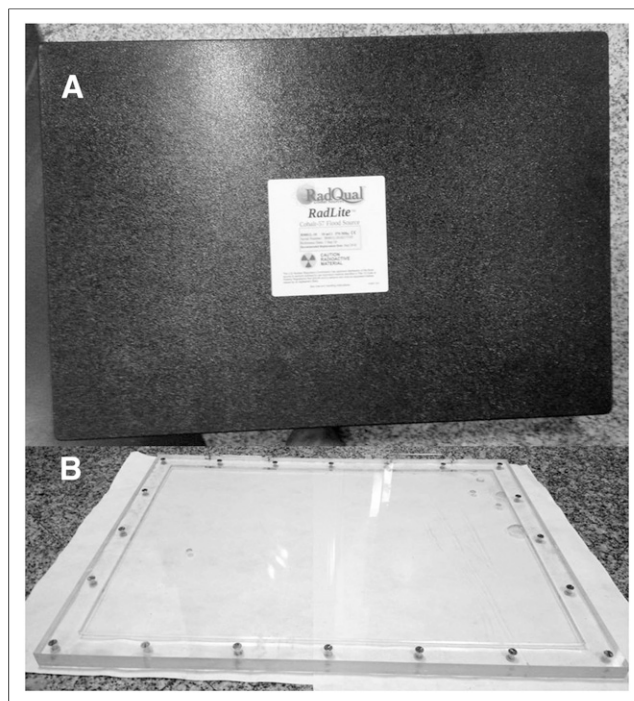
FIGURE 1. (A) Commercially available ^{57}\text{Co} sheet phantom (RadLite; RadQual, LLC). (B) ^{141}\text{Ce} fillable phantom developed in-house by Bhabha Atomic Research Centre.
