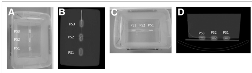
FIGURE 2. Configuration of phantom and point source: photograph showing normal resolution and high resolution (A), fused CT and SPECT images showing normal resolution and high resolution (B), photograph showing metal artifact from lead (C), and fused CT and SPECT images showing metal artifact from lead (D). A color version of this figure is available as a supplemental file at http://tech.snmjournals.org .
