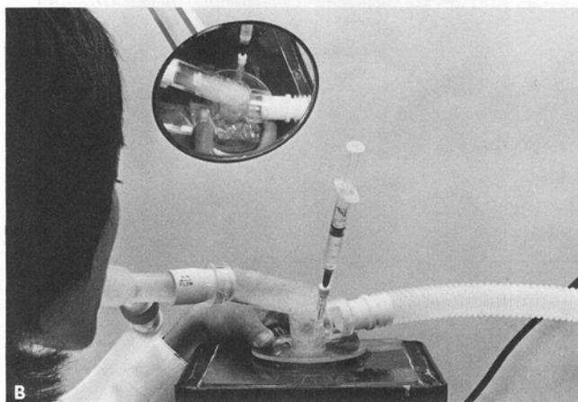
**FIG. 1.** (A) Side view of nebulization chamber. Ring base slides over tapered bottom of chamber, pulling membrane taut over interface. (B) Close-up view of chamber during nebulization.  $^{99m}\text{Tc}$ -phytate is added incrementally through injection inlet.
