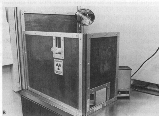
**FIG. 2.** (A) Complete system without shielding. Blower is not capable of opening one-way valves; therefore, system remains closed until patient inhales. Then blower assists movement of aerosol bolus. (B) Shielding effectively minimizes exposure to technologist. Mirror permits technologist to monitor nebulization, and nebulization rate can be adjusted through side opening of shield.
