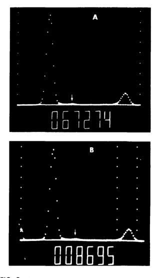
FIG. 2. (A and B) Polaroid photograph of radiochromatogram utilizing 20-cm silica gel plate. Note small peak at Rf.-0.35. Percent free pertechnetate = 16.1%.
