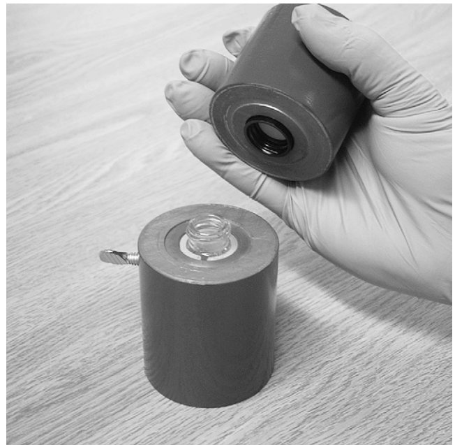
FIGURE 3. Removal of cap from vial and retention of cap in upper section of pig.
