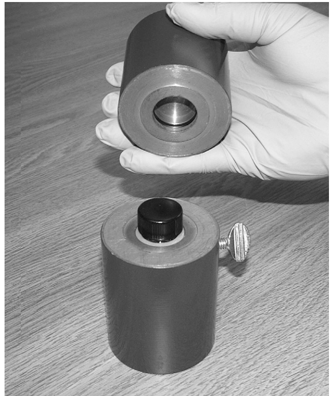
FIGURE 2. Actual placement of screw cap vial in lower section of pig before removal of cap and upper section of pig showing partially recessed O-ring and boss (raised surface).
