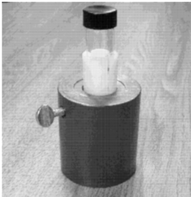
FIGURE 1. Lower section of pig, showing vial, sleeve, and wing nut.
