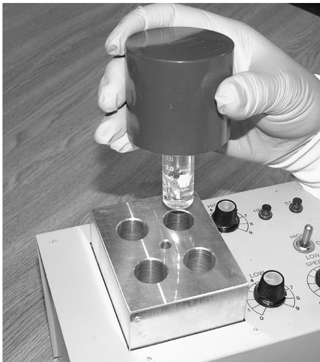
FIGURE 4. Insertion of reaction vial into heating block. In this procedure, top of pig is allowed to remain on vial throughout heating cycle.
