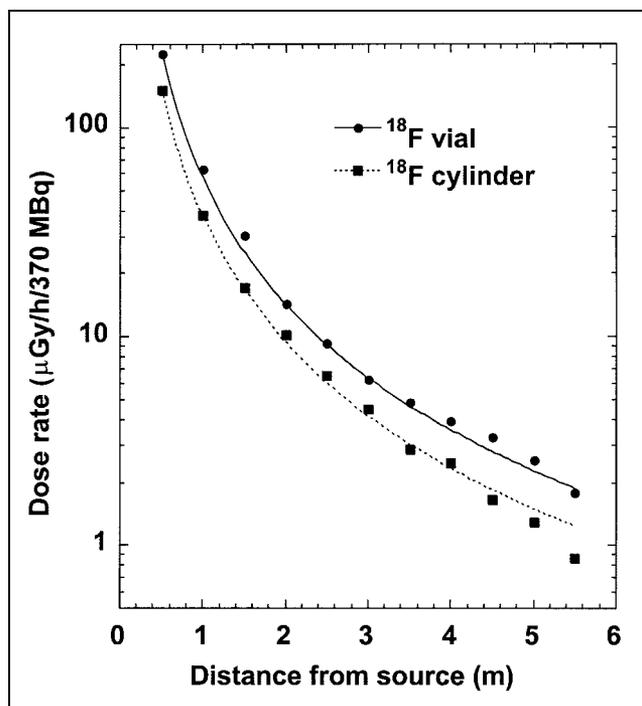
**FIGURE 2.** Dose rates of  $^{18}\text{F}$  vial (● and solid curve) and cylinder (■ and dashed curve) in air as function of distance. Both curves were obtained by fitting to data points using inverse square function. Fitting result is given in Equation 3.
