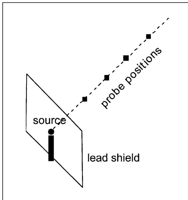
**FIGURE 1.** Experimental setup.  $^{18}\text{F}$  source was placed directly behind lead shield. Dose rates were measured on other side of lead shield at different distances from source using high-pressure ionization chamber.
