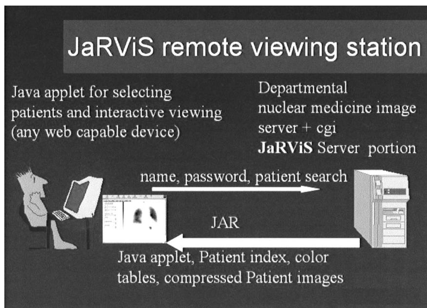
**FIGURE 5.** General scheme for JaRRViS (previously known as JaRViS). *JAR* refers to Java archive, which contains applet and associated files. *cgi* means common gateway interface and refers to small programs that run on server machine, often for handling user interaction.
