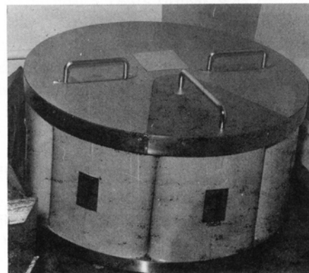
FIG. 2. Cylindrical storage and disposal apparatus containing seven storage boxes for each day of week.
