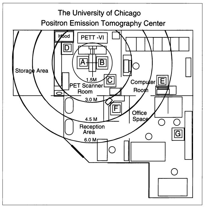
FIGURE 2. A scale drawing of the PET Center at the University of Chicago. The letters indicate the approximate location of the staff involved in a positron tomography study, with the distances from the center of the scanner shown by the circles.
