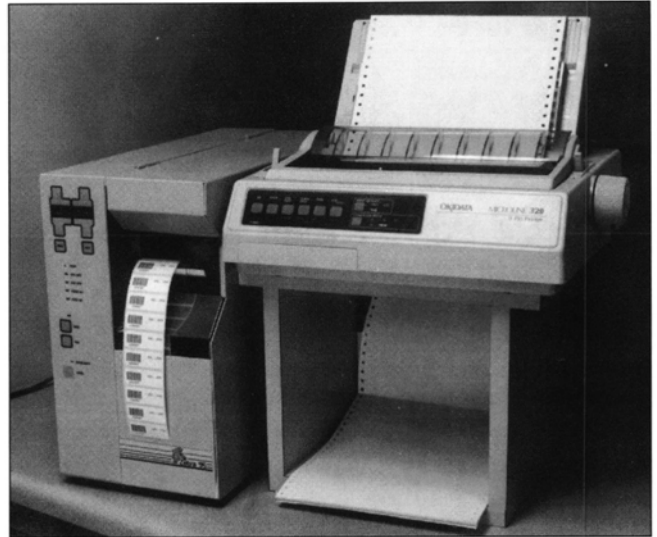
FIGURE 2. The two printers that generate the bar code labels (left) and the daily report (right).
