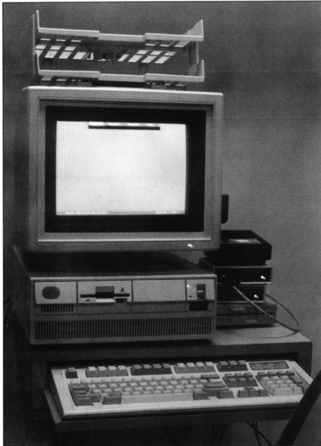
FIGURE 1. The personal computer system with two interconnected bar code readers.
