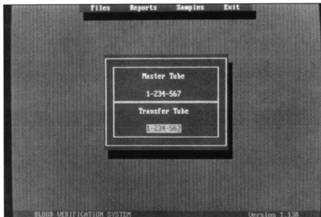
FIGURE 7. Each time the blood product is transferred to a new tube, the bar code on the master tube (i.e., the syringe used to draw the patient's blood) is scanned and compared with the bar code on the transfer tube.
