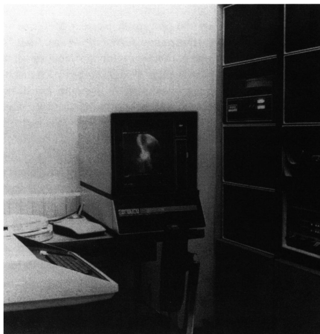
FIGURE 1. DEC GAMMA-11 circa 1970. Notice that software was loaded from paper tape (mid-right) and the user interface was via the keyboard (left) and the joystick (center). The display was a large storage screen.
