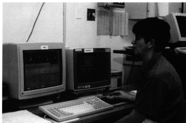
FIGURE 5. Two computer systems are depicted here. On the left is a modern system using the windows interface and the operator is using a mouse to select operations. On the right is the screen for an older, but much modified, GAMMA-11 in which the command structure still prevails as the user interface, but is integrated into the video display screen. The keyboard in this instance is used for both systems.
