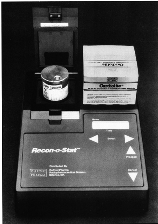
FIGURE 1. Recon-o-Stat thermal controller for the preparation of ^{99m}\text{Tc} Cardiolite and specially constructed tungsten vial shield shown in its operational position mounted on the base.
