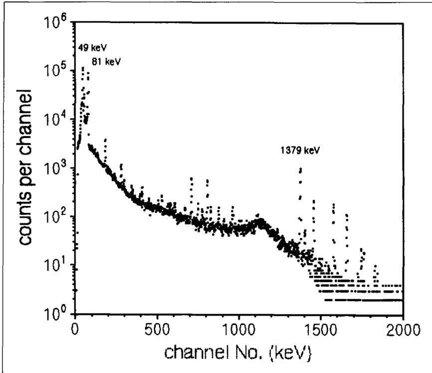
**FIGURE 3.** Typical HPGe spectrum acquired from  $^{166}\text{Ho}$ . The 1.379 MeV photopeak is indicated and other prominent photopeaks detected from  $^{166}\text{Ho}$  are at 49 and 81 keV.
