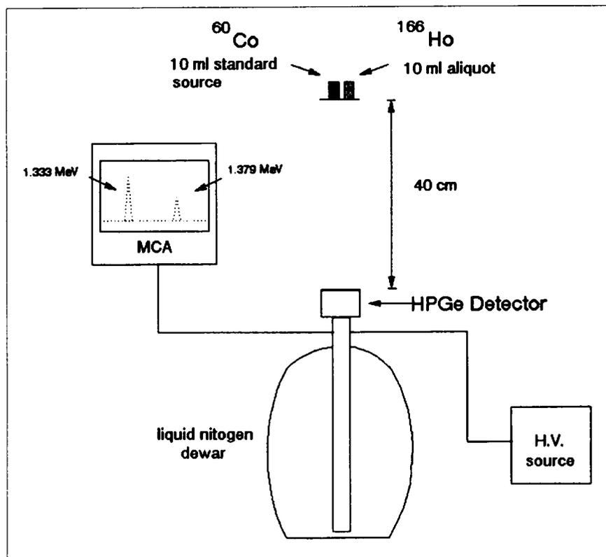
**FIGURE 2.** Diagram of the HPGe detector spectrometer system and location of source at 40 cm from the detector face. A 2048-channel multi-channel analyzer was used for acquisition of all spectra.
