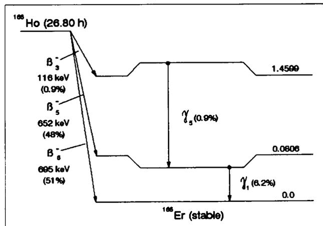
**FIGURE 1.** Simplified decay scheme for  $^{166}\text{Ho}$ . The average energy of each beta particle emitted is expressed in keV. The frequency of the 81-keV and 1.379-MeV photons emitted are given as 6.2 and 0.9%, respectively.
