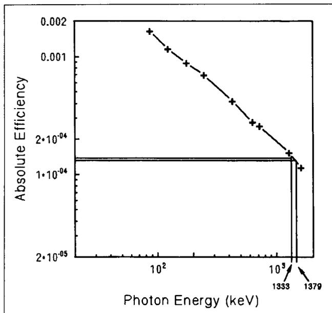
**FIGURE 4.** Absolute efficiency of the HPGe detector efficiency measured with a calibrated NIST mixed radionuclide standard source located at a source-to-detector distance of 40 cm in air.
