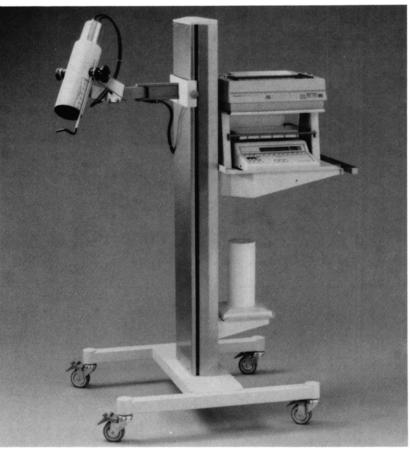
patient and department record keeping. Also included is an automatic calibration mode and a self diagnostic program. The heart of the Atomlab 900 is a microprocessor controlled 256 multi-channel analyzer coupled to a 2" × 2" Nal (Tl) detector. Biodex Medical Systems, P.O. Box 702, Shirley, New York, 11967-0702. (516)-924-9000 ext. 252. Fax: (516)-924-9241.
