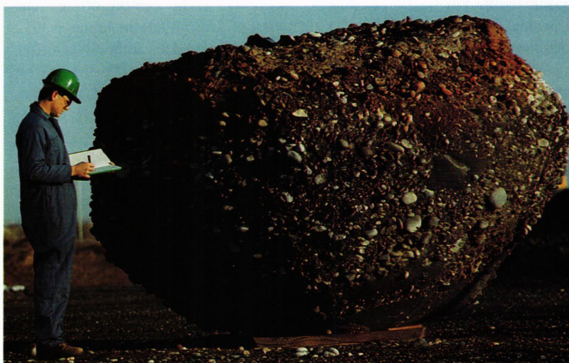
In situ vitrification turns hazardous waste into an obsidian-like mass. Courtesy of Battelle Memorial Institute's Pacific Northwest Laboratories.
