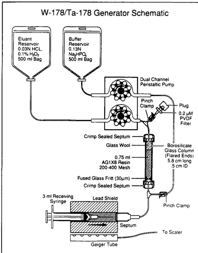
FIG. 4. Schematic of tungsten-178/tantalum-178 generator.
