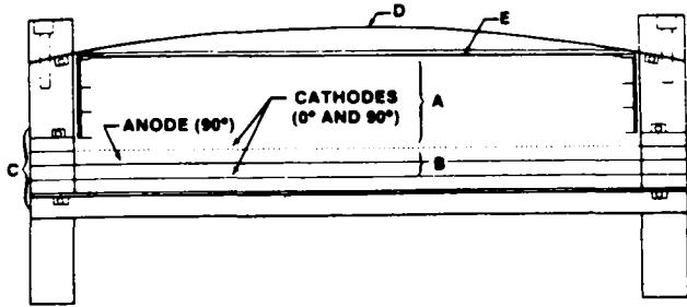
**FIG. 1.** Longitudinal diagram of multiwire gamma camera detector showing: (A) drift region, (B) detection region, (C) aluminum pressure vessel, (D) aluminum entrance window, and (E) negative high-voltage collection electrode.
