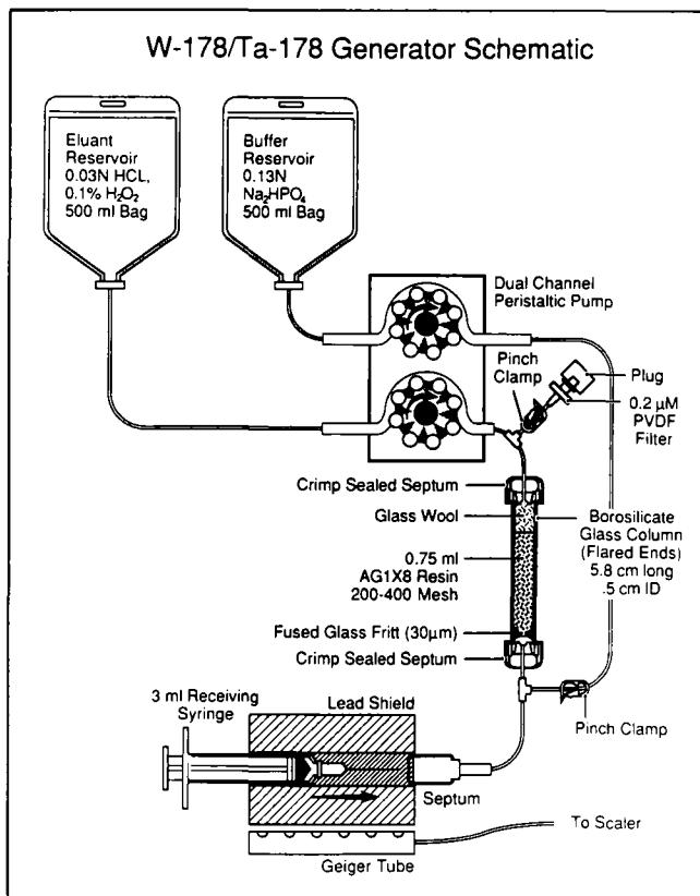
**FIG. 4.** Schematic of tungsten-178/tantalum-178 generator.
