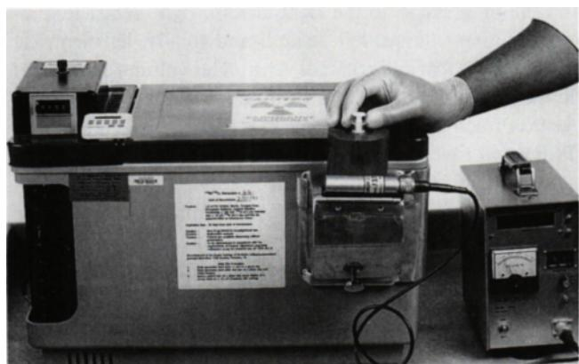
**FIG. 5.** The short half-life of tantalum-178 (9.3 min) makes it necessary to have a portable generator, which can be eluted at bedside.
