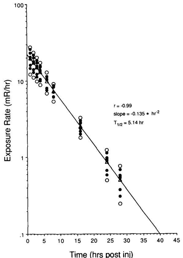
**FIG. 1.** Exposure rate at skin surface over kidney plotted against hours postadministration of technetium-99m DTPA. Mean exposure rate is represented by triangles and s.d. of  $\pm 2$  by open circles. Individual readings from each study are presented as scatter plots (closed circles).
