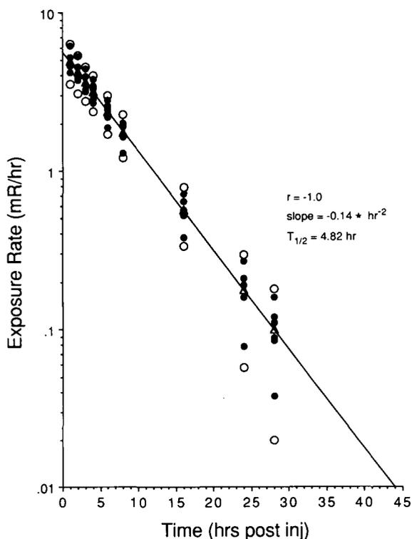
**FIG. 2.** Exposure rate at one foot from skin surface over kidney plotted against hours postadministration of technetium-99m DTPA. Mean exposure rate is represented by triangles and s.d. of  $\pm 2$  by open circles. Individual readings from each study are presented as scatter plots (closed circles).
