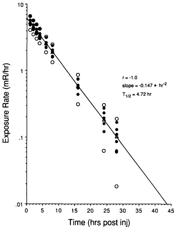
**FIG. 4.** Exposure rate at one foot from skin surface over bladder is plotted against hours postadministration of technetium-99m DTPA. Mean exposure rate is represented by triangles and s.d. of  $\pm 2$  by open circles. Individual readings from each study are presented as scatter plots (closed circles).
