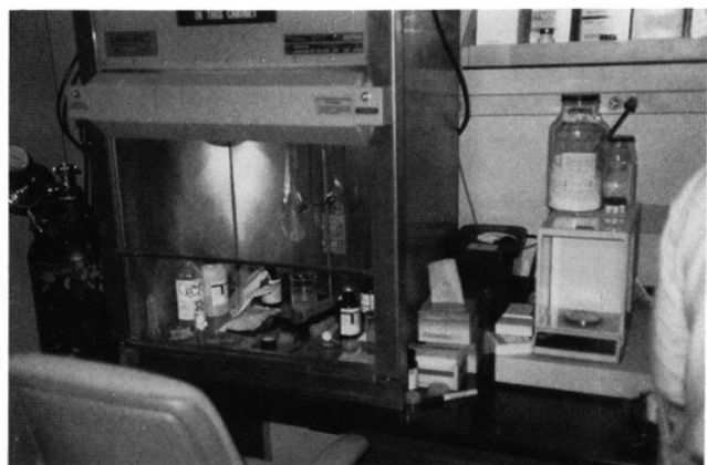
FIG. 5. (A) A laminar flow hood set up for dispensing PET radiopharmaceuticals. Note the reinforced base and lead bricks. (B) A small laminar flow hood provides a clean environment for the preparation of radiopharmaceutical synthesis apparatus.
