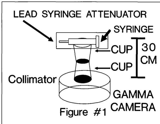
**FIG. 1.** Two large styrofoam cups glued together at their bottoms are used to elevate and support the lead shield attenuator to 30 cm above the collimator surface.
