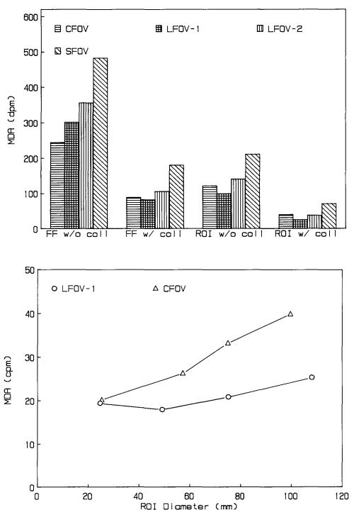
FIG. 1. Minimum detectable activity in dpm for four cameras. MDAs were determined as follows: FF w/o coll full field without collimator, FF w/ coll—full field with collimator, ROI w/o coll—region of interest without collimator, and ROI w/ coll—region of interest with collimator.
