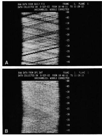
**FIG. 3.** Sinogram display of a daily QA emission scan (ES) having a bad detector present, apparent as a black line in (A). The sinogram following correction of the data set using interpolation and detector inhomogeneity correction is shown as (B).
