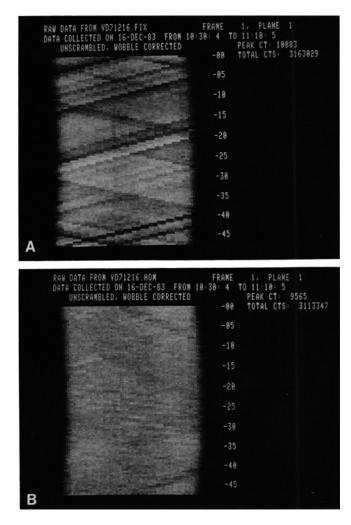
FIG. 2. Sinogram displays of a typical daily QA ES shown (A) before any corrections are applied, and (B) after detector inhomogeneity correction is applied. Note the marked improvement in the uniformity of the response in the data set.
