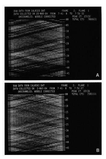
**FIG. 1.** Sinogram displays of EPS obtained (A) before detector adjustments performed as preventive maintenance, and (B) after detector adjustments performed as preventive maintenance.
