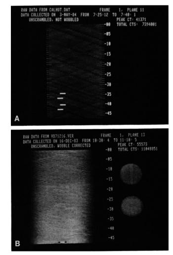
**FIG. 5.** Sinograms illustrating problems producing only subtle visual artifacts in the daily QA images. Note that these artifacts are strikingly apparent in the sinograms. They arose from a software problem during some transmission rod source data collections. Both artifacts were correctable using specialized software interpolations on the raw data sets.
