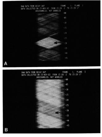
FIG. 4. Sinograms illustrating two PET camera problems, which occurred during high count rate QA tests. They correspond to problems with (A) coincidence gain ICs and (B) a data acquisition coincidence board.
