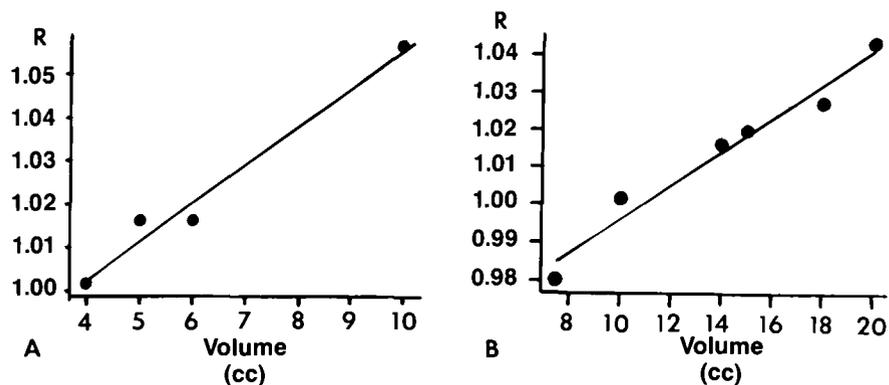
FIG. 1. Geometrical variation of the  $^{99m}\text{Tc}$  assay between the retractable canister and the standard method. Activity ratio (R) as a function of elution volume (cc). (A) 10-cc vial and (B) 20-cc vial.
