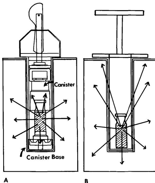
**FIG. 4.** Assay geometry for the  $^{99m}\text{Tc}$ . (A) Retractable canister and (B) standard canister.
