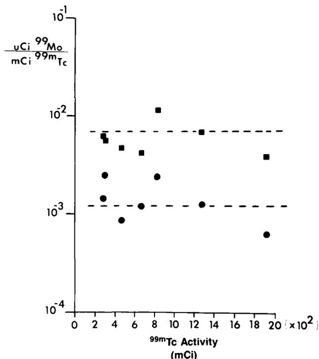
**FIG. 3.** Molybdenum-99 contamination level measured by the commercial canister ● and the standard canister ■.
