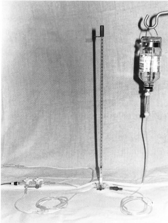
**FIG. 7.** Cystometric calibration system. Transducer connected via 2 gang stopcock to manometer which measures up to 40 cm of water.
