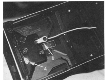
FIG. 6. Camera back pressure plate indicating the solder point contact (A) and solder lug (B).
