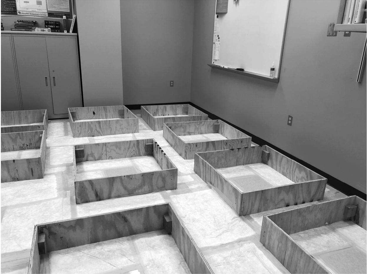
**Figure 1: 3ft<sup>2</sup> Plywood Sample Boxes and Absorbent Pads Ready for Controlled
