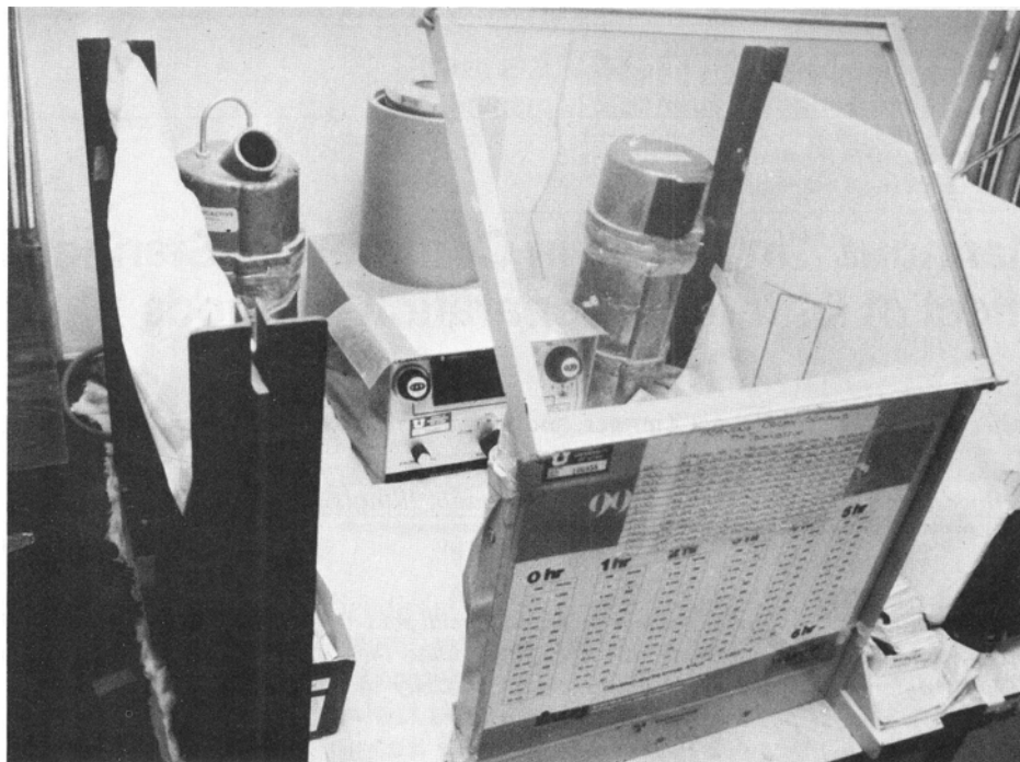
FIG. 4. Drawing station surrounded with ¼ in. lead shields supported by a brace of angle iron. Note waste containers located on either side of dose calibrator.
