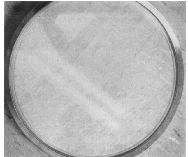
FIG. 5. Crystal originally damaged by thermal shock results in pattern of regular wide-spaced cracks shown in upper half. Subsequent careless handling produced more intense mechanical damage pattern in lower half.
