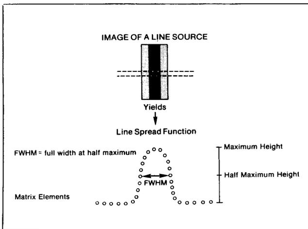
**FIG. 2.** Diagrammatic representation of the line-spread function.
