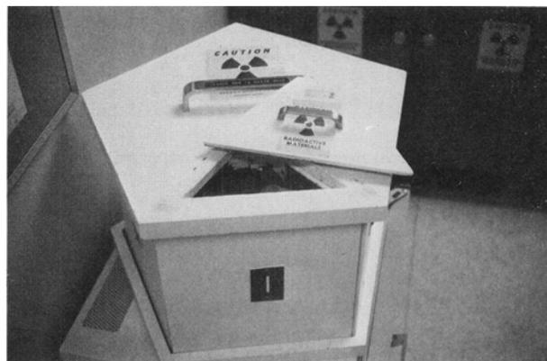
**FIG. 1.** Five-Compartment hot trash unit for day-of-the-week storage and decay. Access door is lead lined; top is easily positioned to reveal other compartments.
