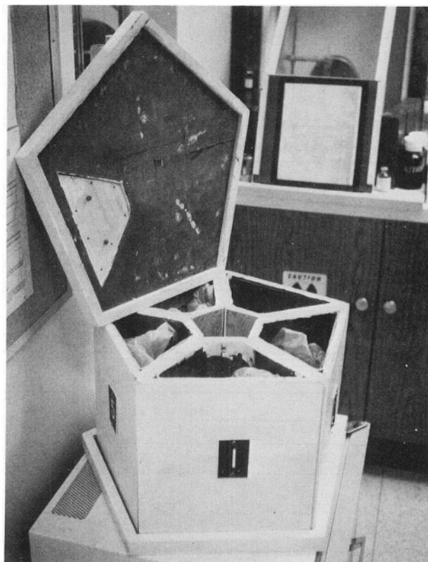
**FIG. 2.** Top of structure raised shows five separate areas for waste storage. Six- and seven-compartment units are conceivable.
