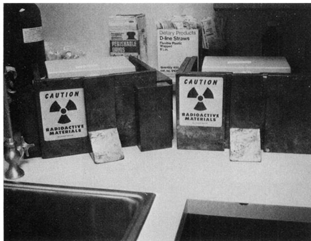
**FIG. 3.** Conventional method of generator setup; front lead piece is removed for elution vial placement.
